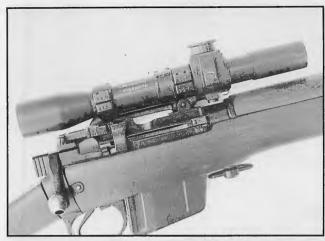
Optical equipment for the L42A1 consists of the World War II No. 32 Mk III 3X scope and mount rebuilt and regraduated for the 7.62x51mm cartridge with 144-grain bullets and redesignated as the "Telescope Straight Sighting L1A1."
